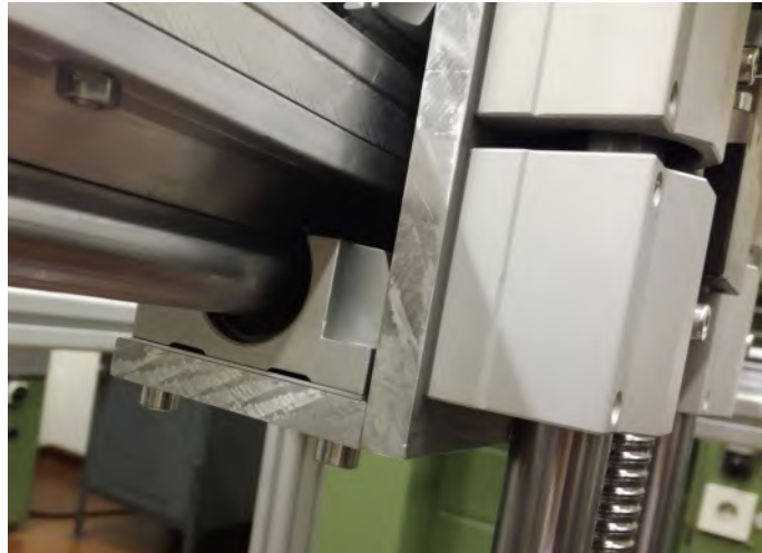
Figure 31: Close up of the attached axis. Please note that a distance plate of 1mm thickness has been used at the bottom for an improved fit.
