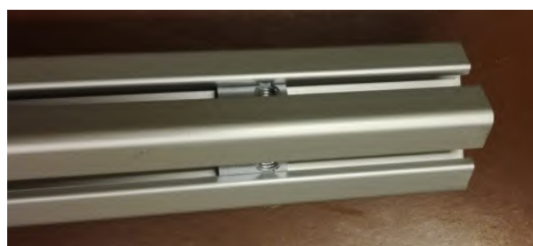
Figure 8: Inserted slot nuts at each end
