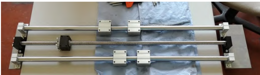
Figure 24: Assembled bearings of the Easy-Mechatronics system with the aluminum plates 8 & 9.
