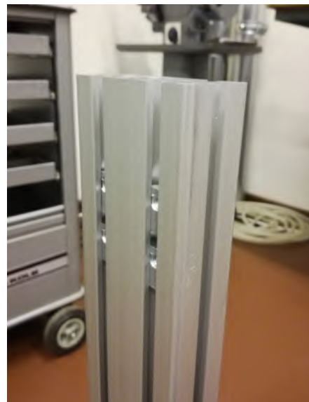
Figure 11: “Right” side 4 slot nuts
