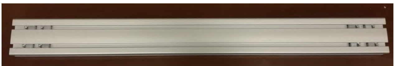
Figure 3: Slot nuts inserted in aluminum frame
