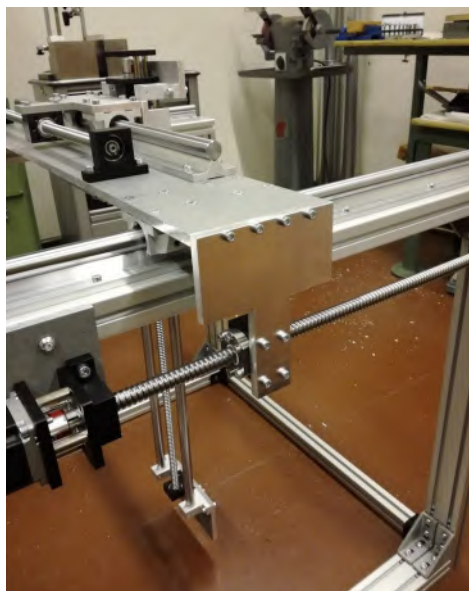
Figure 33: Attached plate 2, plate 1 and the ballscrew block from the x-axis.
