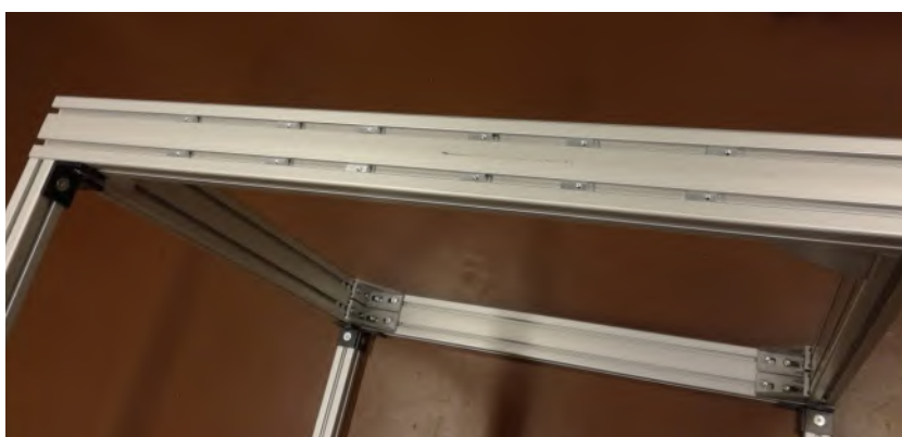
Figure 19: Inserted slot nuts at one side of the structure
