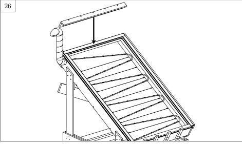
Place the upper part of the cover on the upper part of the pane, so that the damping lies on top of the glass pane. It has to be installed centrally. The glass needs some space to expand otherwise it will break. It needs at least 0.2" distance to the cover.
