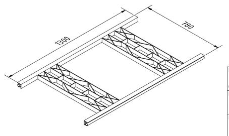
All parts are welded. Note: All units in mm.
