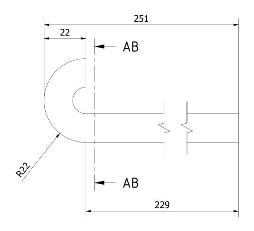
Note: All units in mm. CREATED BY APPROVED BY PROJECT 31/08/2021 Scooter with fat tire PART NAME J. Rosciano A. Morillo 1.2 POS 2.16 QUANTITY Pin.ipt Pin DEVELOPED BY REDESIGNED BY DOC. TYPE MATERIAL Part LICENCE DIN C45 SCALE SHEET 34 /65 OHO e.V. 1/1 ОНО CC-BY-SA 4.0
