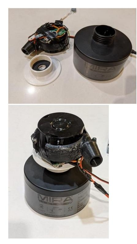
This is an adapter plate for a 3M P100 or N95 face mask filter cartridge. These are more commonly available than the above filters. The brown rubber washer is pulled from a 3M mask. Download [3D model] [Fusion 360 link]
