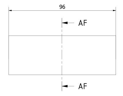
Note: All units in mm. APPROVED BY PROJECT CREATED BY Power Hammer Krusty 31/08/2021 J. Rosciano A. Morillo 1.1 POS PART NAME Anvil B.ipt 5.6 QUANTITY Anvil B DEVELOPED BY REDESIGNED BY DOC. TYPE MATERIAL Steel 4130 Part LICENCE SHEET 42 /75 OHO e.V. 1/1 **KROMM Steel Works** CC-BY-SA 4.0
