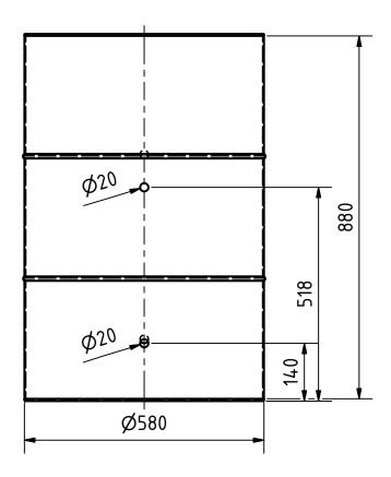
NOTE: holes alligned to inner tank tubes
