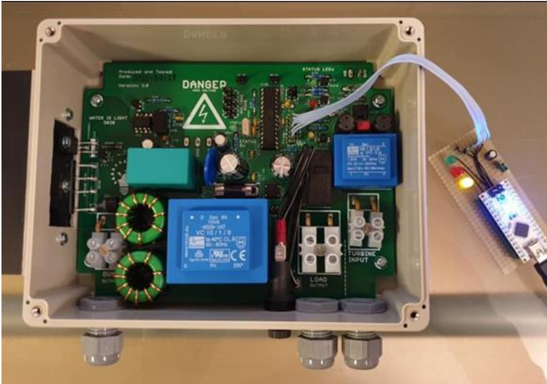
WIL Turbine construction 6: ELC construction October 12, 2022
