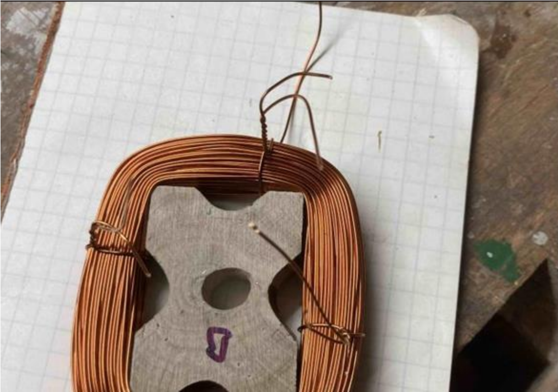
WIL Turbine construction 4: Sgulen winding August 20, 2022
