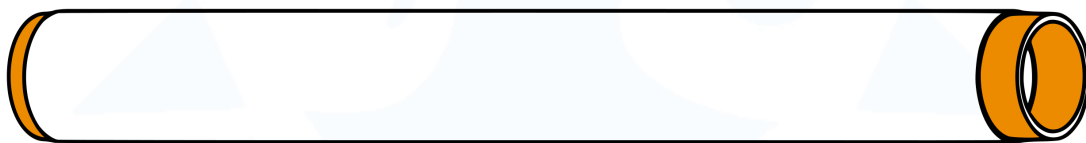
Fig. A.31.: The ends of the connection pipe’s inner and outer diameter need to be adjusted on a lathe. The fit on these parts has to be very tight.
