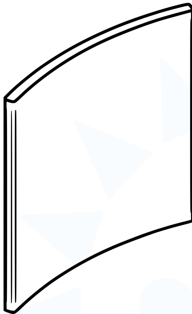
Fig. A.18.: The vanes guide water inside the flow channel
