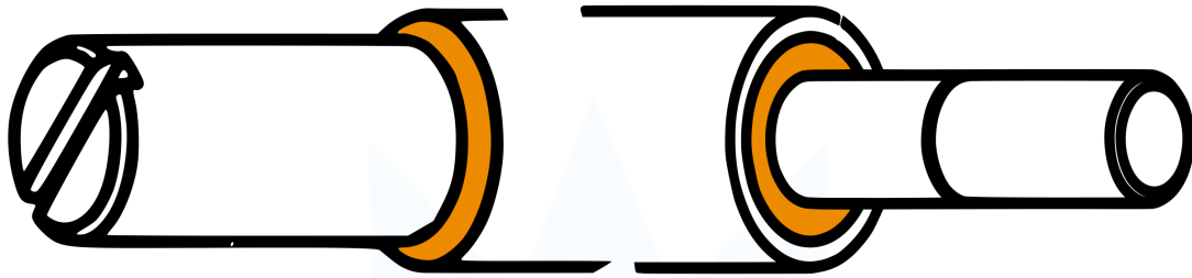
Fig. A.41.: Weld the two thread shafts onto the shaft
