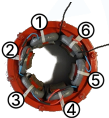
Fig. A.50.: Finished wiring of the coils (numbered)
