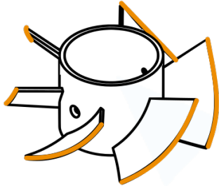
Fig. A.28.: Turn the propeller to the specified diameter
