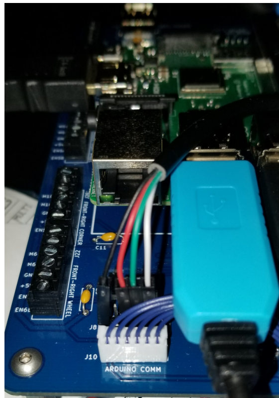
Figure 5: USB / TTL Serial Cable Connection
